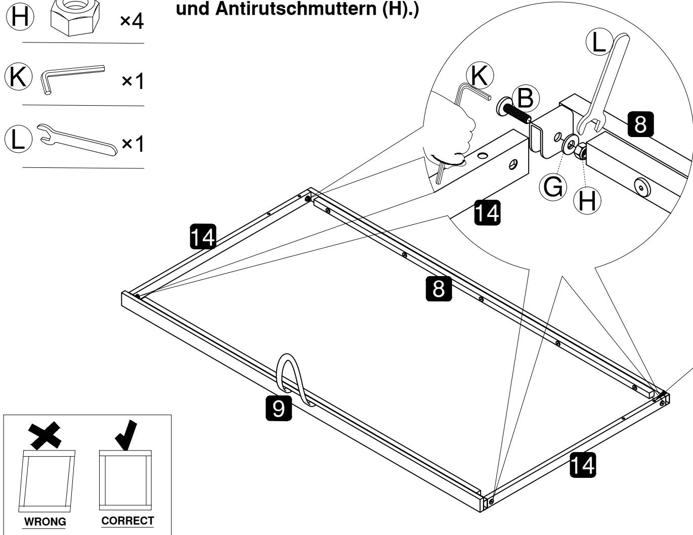
Note the position of the rear bed beam (8) of the traction bed and the front bed beam (9) of the traction bed, as shown in the figure: The rear bed beam (8) of the traction bed is located at the screw hole end of the front tube (14) of the traction bed.
