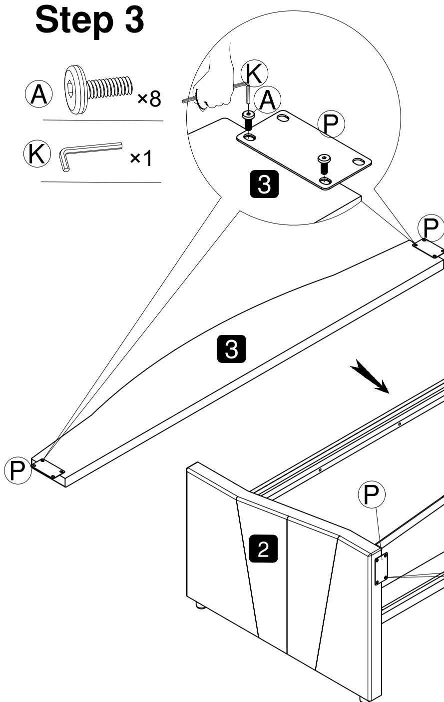
Use the hexagonal wrench (K) to fix the backrest (3) to the armrest (1)&(2) with bolts (A).
