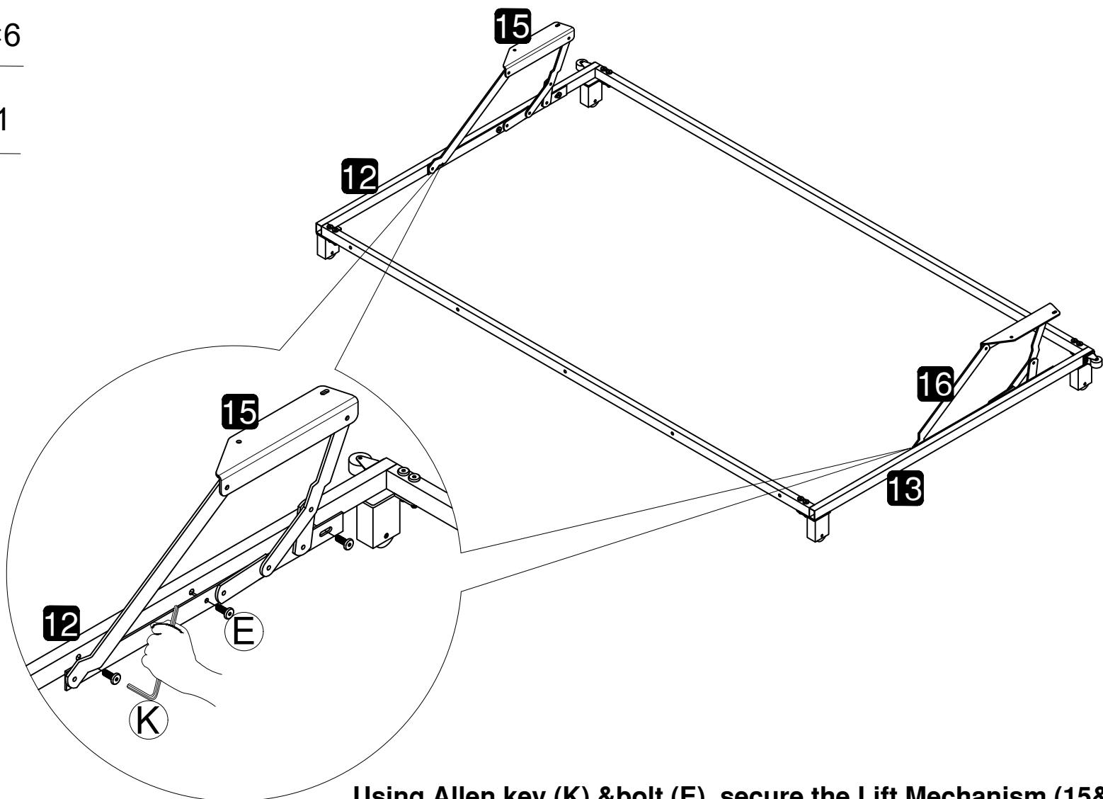
Using Allen key (K) & bolt (E), secure the Lift Mechanism (15&16) to the Tow bed side pipe (12&13).
