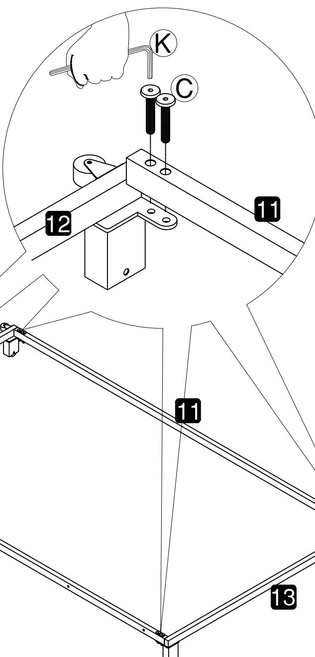
Using an Allen key K&bolt C, connect the Tow bed front tube (10)&To bed rear pipe (11) to the Tow bed side pipe (12&13).
