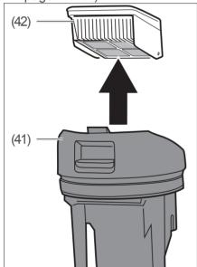
3. Pull the filter element (42) out of the wastewater tank cover (41).
