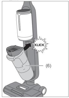
3. Insert the wastewater tank bottom first into the appliance and then push the top of the wastewater tank onto the appliance until the tank audibly clicks into place.
