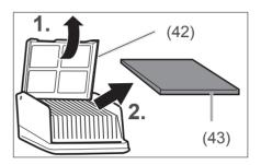
4. Open out the filter element and remove the HEPA filter (43).
