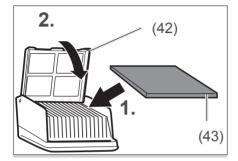
1. Place the HEPA filter (43) in the filter element (42) and close the filter element.
