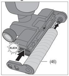
Slide the brush roller (46) sideways onto the mount. As you do so, orientate the brush roller so that the brush roller release (13) clicks into the holder.
