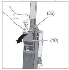
Remove battery compartment cover (10): Press the release button (35) and remove the battery compartment cover.
