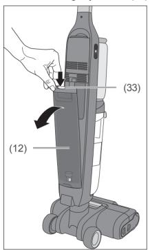
Grip the appliance firmly with one hand. With the other hand, take hold of the fresh water tank (12) and press the release button (33) downward. 2. Pull the fresh water tank out of the appliance.
