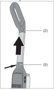
Using a pointed object such as a screwdriver, press the handle release (9) and pull the handle (2) out.
