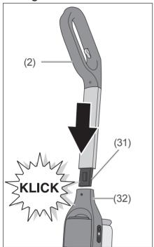
Slide the joint section (31) on the handle (2) into the slot on the appliance (32) until it audibly clicks into place.
