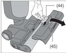
2. Pull the release handle (44) of the brush cover (45) upwards to remove the brush cover
