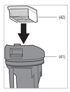
2. Insert the filter element (42) into the wastewater tank cover (41).
