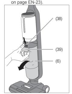
2. Grip the appliance firmly with one hand. Hold the wastewater tank handle (39) with the other hand and press the release button (38) down with your thumb. 3. Pull the wastewater tank (6) out of the appliance.
