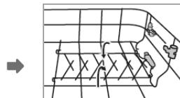
To create a better arrangement for bulky dishes, the rack shelves can be folded. Lift the racks slightly and fold them down.
