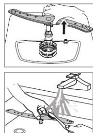
Lime and impurities from the rinsing water can block nozzles and bearings of the spray arm. Check the outlet nozzles of the spray arm regularly for blockages.
