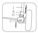
4.Press the fragment (K), respectively insert the backwheels sets into backfoot tube's two sides(I).Push up the fragment (K) of backfoot tube popup from the back seat plastic hole.Ensure the wheel sets do not fall out means the installation completed. When you need to disassemble wheel sets, press the fragment and pull down the wheel seat.When you do not need push stroller,you should step down back brake lever(C)then the
