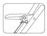
3. When baby sleeping ,you can pull the legrest to extension seat's length. When baby need to sit ,push down two sides buttons then the legrest can be laid down.
