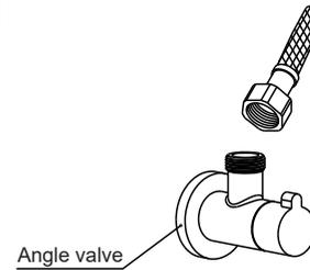
1. Connect the inlet hose to the angle valve according to the hot and cold mark and tighten. Before connecting, please confirm that there is a sealing rubber gasket in the inlet hose connector.
