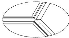
**Note:** Before tightening, must align the slots on the poles and the top frame.
