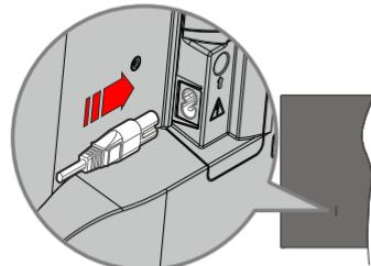
Plug one end (the two-hole plug) of the supplied detachable power cord into the power cord inlet on the rear side of the TV as shown above. Then plug the other end of the power cord into the mains socket outlet.
