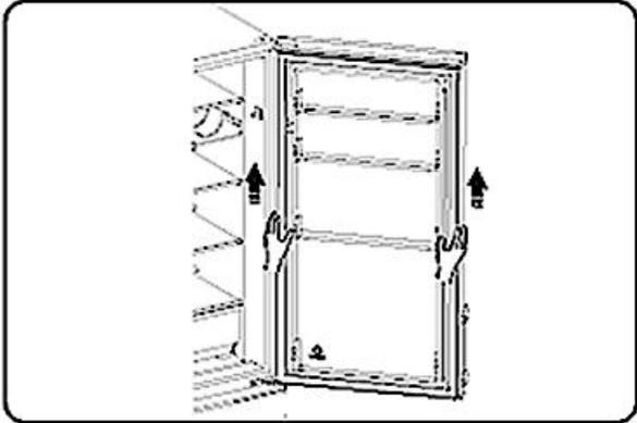
8. Remove the door stop block (4) and the door bearing bush (5) from the left-hand side of the appliance door and reinstall them on the right-hand side of the door (s. fig. below).
