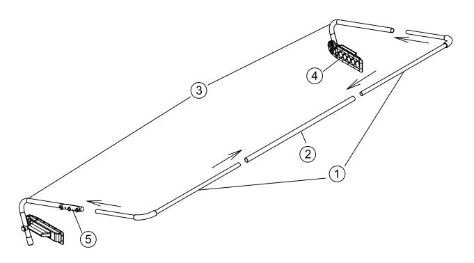
Installation steps One: Install the stents on both sides respectively
