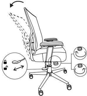
**English:** Rocking function can be adjusted to 10° in 2nd gear and 15° in 3rd gear. Take care to slowly adjust the angle you need.
