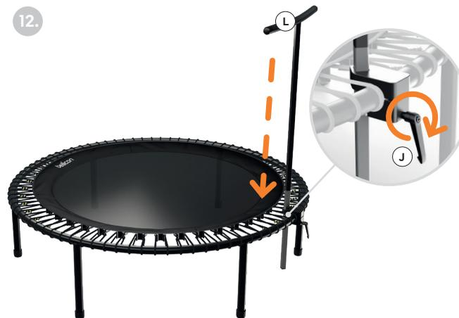
**EN:** Place the bellicon on all six legs. Push the T-bar (L) from above through the square hole so that the handle of the T-bar is parallel to the frame of the bellicon. Adjust the T-bar to your desired height and tighten the clamping lever (J).
