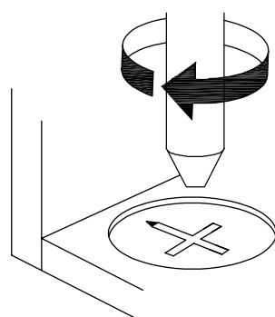
**EN**\_Turn cam lock clockwise to tighten.
