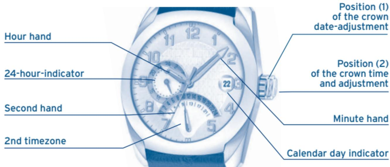
Adjust crown to position 2 (Pull right out).
