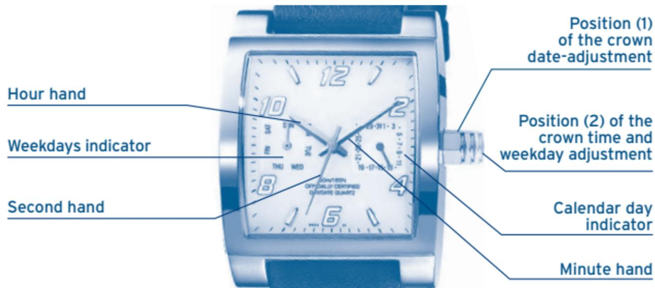
Adjust crown to position 2 (Pull right out).
