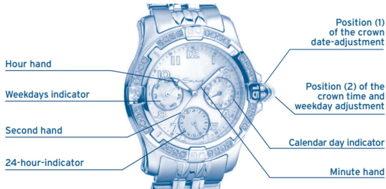
Adjust crown to position 2 (Pull right out).
