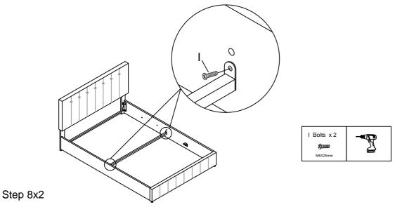
Fix the gas lifts  $\bigcirc$  to the side rails  $\bigcirc$  with blots I by using electric drill.fix the gas bar to the gas lifts  $\bigcirc$  with nuts H
