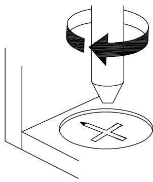
**EN**\_Turn cam lock clockwise to tighten.
