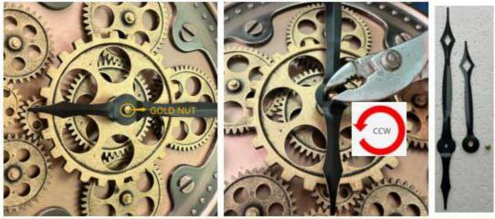
Step 3: Aligning to 12 O'clock, insert hour hand into shaft(slightly press the middle to fit the shaft), then insert minute hand and screw nut cap back. Keep both hands parallel and turn two full cycles to ensure the hands are not touching each other.
