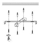
Drill holes & apply plastic anchors With screws
