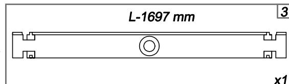
**(GB)** Install the beam no 3 on the 4th layer. If pool installed in area where temperatures fall below 0°C , install the beam no 3 on higher layer.
