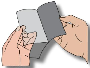
Remove the protective film by approx. 5 cm and fold over.
