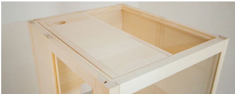
Fig. 14: Inserting front ceiling element
