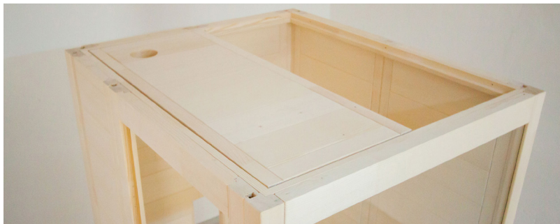
Fig. 14: Inseting the front ceiling elements
