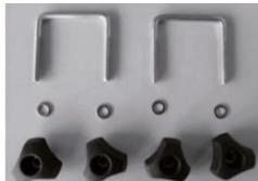
Now feed one U-shaped bracket, from below, through the drilled holes of the base plate. Fit the washers and knob nuts to the threads of the U-shaped bracket. Tighten the nuts gently. Do the same on the other side.
