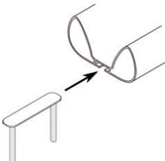
Fit the end caps onto the ends of the wheel rail.
