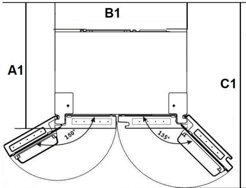
**A 1 = Depth / B 1 = Width / C 1 = Depth (when the door is open)**
