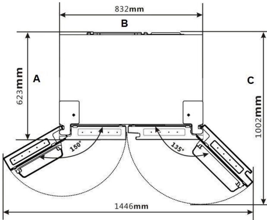
**A = DEPTH / B = WIDTH / C = DEPTH (WHEN THE DOOR IS OPEN)**
