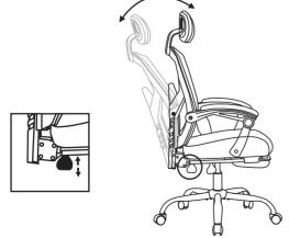
While seated, reach the right side of the chair to find the handle at back. Lift it up to horizontal direction and lean your body back slowly, push the handle down until the desired tilt angle is reached. Lift the handle up and move your body away from the chair back slowly to restore the backrest to the vertical angle.
