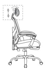
Move the headrest up/down to adjust the height to the desired height. Angle the headrest up/down to the desired position.
