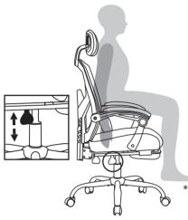
While seated, reach the right side of the chair to find the handle at front. Lift it and raise your body up slightly to allow the chair to rise to the desired height. To lower the seat, lift the handle while applying more weight downward on the seat. The chair will descend until the handle is released or the chair reaches the bottom position.
