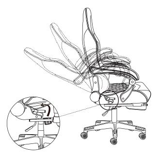
Pull the lever FULLY and lean back slowly until desired angle is achieved, then slowly return the lever to its starting position Ensure the lever locks back in place.
