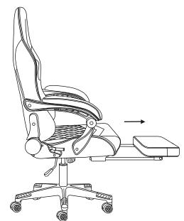
Pull out the pole of the footrest, and turn the footrest to the front.
