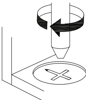
**EN\_**Turn cam lock clockwise to tighten.
