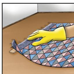
4. Align the edges of the element you would like to attach so they are in line with the tape. Place the element on the tape and press down firmly for a few minutes.
