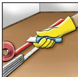
2. Measure the tape to the desired length and cut it off.
