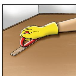
3. Place the tape (adhesive side downward) on the surface and press firmly. Remove the red protective film from the tape.
