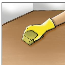
1. Clean the surface to which the tape will be applied from oil and dirt. The surface should be clean, dry and not too rough in order to achieve an optimum adhesion result.
