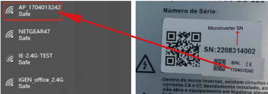
Microinverter SN: 2208314002 Built-in datalogger :1704013242
