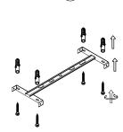
Drill holes & apply plastic anchors With screws
