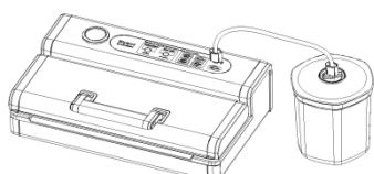
Insert one end of the hose into the hose port and another end of the hose into the center hole of the canister cover.
