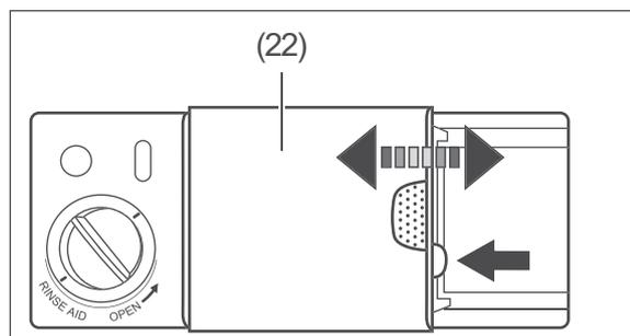
1. Push the blue fastener of the compartment for dishwasher detergent/multitabs (22) to one side. The cover will move to one side and the compartment will become visible.
