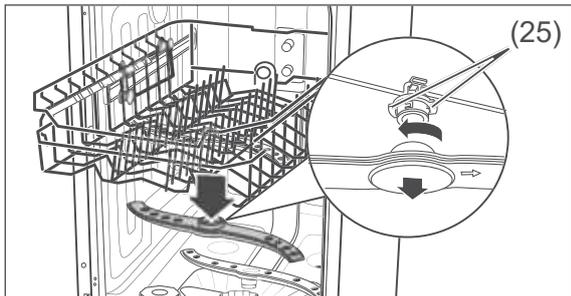
3. The upper wash arm is attached by means of a bayonet fitting. To remove the spraying arm, hold the two serrated bayonet grips (25) still and turn the spraying arm clockwise.
