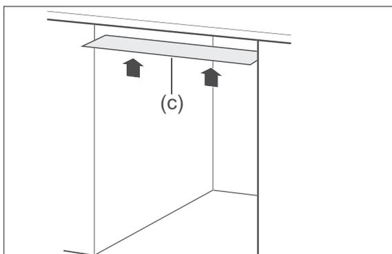
3. Affix the enclosed condensation-protective film (c) to the bottom of the work surface. In this way, you will avoid damage to the worktop as a result of hot steam which may come out of the dishwasher when the door is opened.
