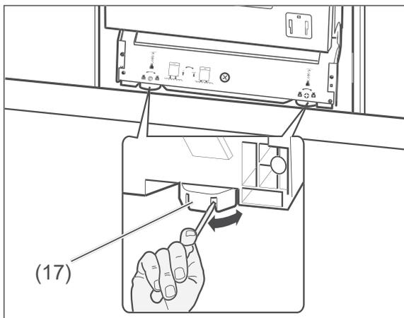
8. To position the dishwasher so that it is level, the two front adjustable feet (17) and the back adjustable foot of the appliance can be adjusted by up to 50 mm.
