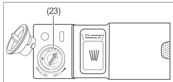
1. Turn the cover of the dishwasher salt compartment (23) a quarter turn in an anti-clockwise direction and remove it.
