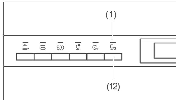
2. Hold the (12) button down until the display shows the current hardness (H1 to H6).
