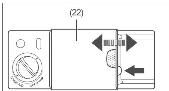
1. Push the blue fastener of the compartment for dishwasher detergent/multitabs (22) to one side. The cover will move to one side and the compartment will become visible.
