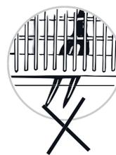
When loading the cutlery, ensure that the cutlery does not go through the bottom of the cutlery basket. Otherwise, the lower spraying arm will be blocked.
