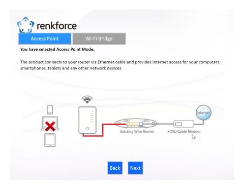
**2.** Connect the network port of your EW-7476RPC to the LAN port of your existing router using an Ethernet cable, then click "Next".
