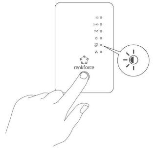
**3.** The devices will establish a connection. The extender's **green** WPS LED should display on for 30 seconds to indicate a successful connection.
