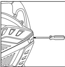
4. Loosen the fan cover screw counterclockwise, the screw should remain on the cover.
