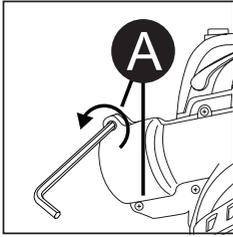
1. Remove the screws (A) on the drive head with the Allen key provided and store them in a safe place.
