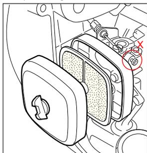
Allow the unit to idle. Adjust the idle speed so that the machine runs without stopping (idle speed too low).
