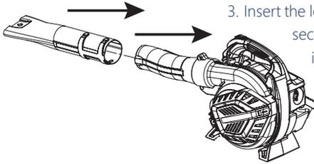
3. Insert the lower blower tube into the upper blower tube and secure it with the 2 screws. To disassemble, proceed in reverse order.
