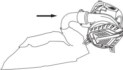
3. Insert the end of the connecting tube into the drive head housing and then push it towards the machine. Tighten the screws again.
