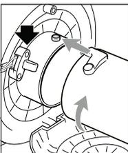
6. Lower the fan cover and insert the upper suction tube. Make sure the contact plate is aligned with the safety switch on the head. Push the tube in as far as it will go, then turn it counterclockwise.
