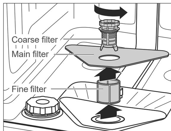
Check the coarse filter, the main filter and the fine filter after each rinse cycle and remove food residues and foreign bodies if necessary.
