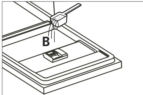
3. Pour the remaining 1/5 of the dishwasher detergent inside the appliance door **B**. Your appliance uses this quantity during the pre-wash programme.
