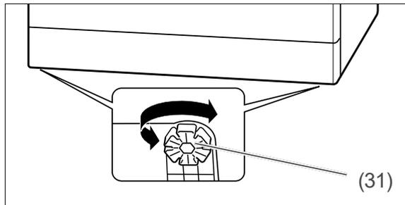
5. In order to compensate for uneven floor surfaces and set up the dishwasher on a level horizontal base, you can screw the four adjustable feet (31) in or out. The adjustable feet have slots around their circumference. Insert a screwdriver and turn the adjustable foot. Use a spirit level to set up the dishwasher.
