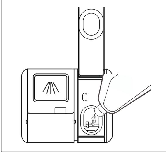
2. Fill the water tank to the “max” mark in the opening.
