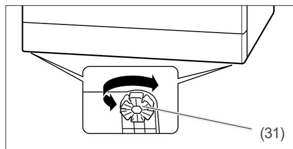
3. In order to equalise unevenness in the floor and set up the dishwasher on a level horizontal base, you can screw the four adjustable feet (31) in or out. The adjustable feet have slots around their circumference. Insert a screwdriver into one of them and use it to turn the adjustable foot. Use a spirit level to align the dishwasher.
