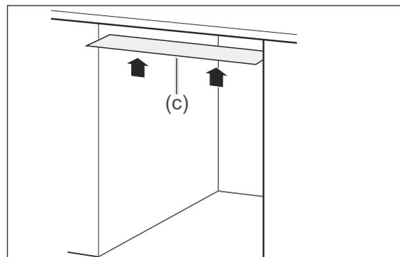
3. Affix the condensation protection film supplied (c) to the underside of the worktop. In this way, you will avoid damage to the work surface as a result of hot steam which may be emitted from the dishwasher if the appliance door is left open.
