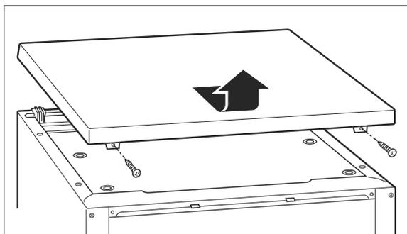
2. Loosen both screws on the reverse side of the covering panel and remove them.
