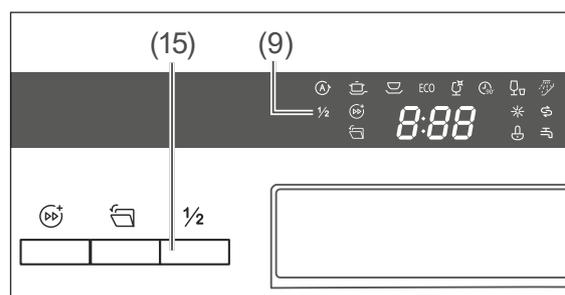
Select the “Half load” option if you would like to run the appliance with less than 6 place settings. This additional option reduces water and power consumption.
