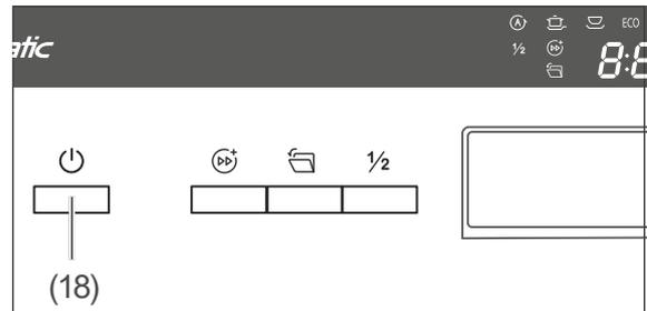
3. If the dishwasher is switched on, switch it off with the  $\odot$  button (18).
