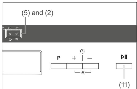
2. Press and hold the **P** button (13) until the  $\ast$  indicator (5) and the  $\odot$  indicator (2) flash alternately.
