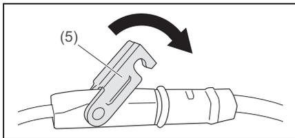
2. Fold the latch (5) down to securely lock the plug connection.
