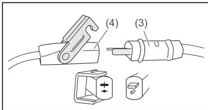
1. Insert the plug (3) into the jack (4). The form of the contacts prevents any reversal of polarity.
