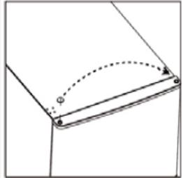
A technical drawing showing the cap being applied to the right side of the door. A dashed line indicates the door being lifted from the bottom hinge and swung to the side.         |
