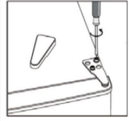
A technical drawing showing a hand using a screwdriver to pry off a triangular cap from the top hinge of a door. The cap is shown separately to the left.                             |
