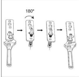
A technical drawing showing the process of rotating the hinge. A pin is removed from the hinge, the hinge is rotated 180 degrees, and the pin is reinserted into the opposite side. |
