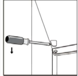
A technical drawing showing a hand using a screwdriver to pry off a cap from the left side of the door's hinge mechanism. A downward arrow indicates the direction of removal.        |
