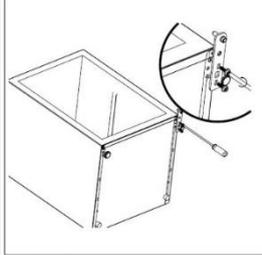
A technical drawing showing the device being tilted back. A hand is shown using a screwdriver to unscrew the bottom hinge from the right side of the device.                        |
