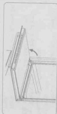
2. Open the locking catch (a) (with the aid of a screwdriver) up to the end position.
