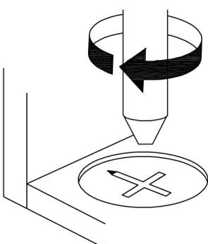
**EN**\_Turn cam lock clockwise to tighten.
