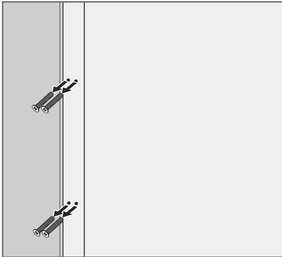
1. Unscrew the four screws from the side of the appliance door (3).
