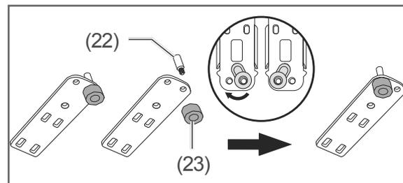
4. Detach the hinge pin (22) and the support foot (23) from the lower hinge.
