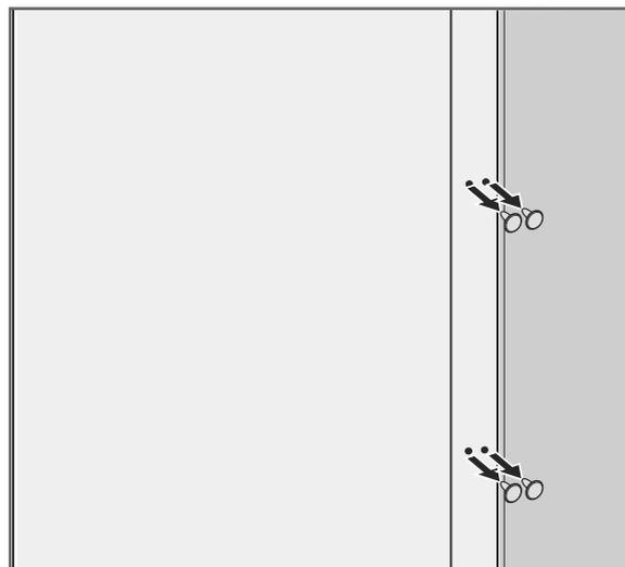
4. If you wish to fit the door handle on the opposite side after changing the door hinge, you must first remove the blind plugs.
