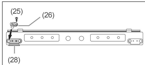
4. Screw down the plastic insert (26) on the opposite side of the appliance door.
