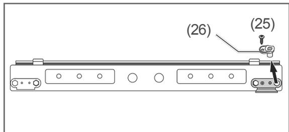
1. Loosen the screw (25) and remove the plastic insert (26).
