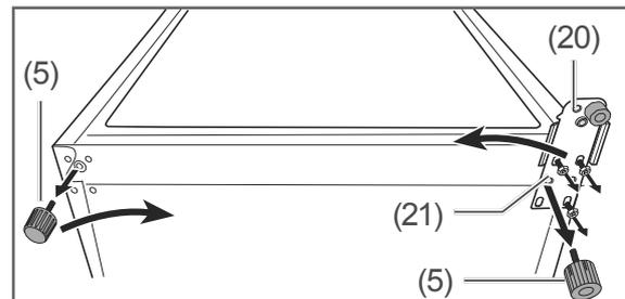
2. Loosen the screws (21) on the lower hinge (20).
