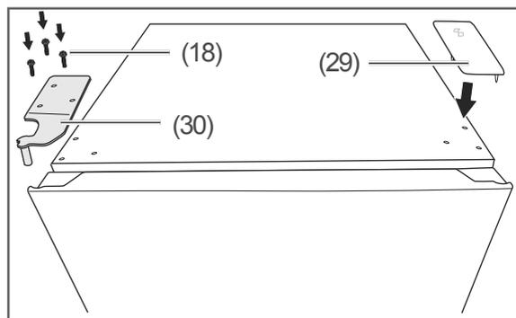
1. Tighten the upper hinge (30) with the screws (18).
