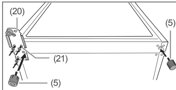
7. Fasten the lower hinge (20) on the left side with the screws (21).
