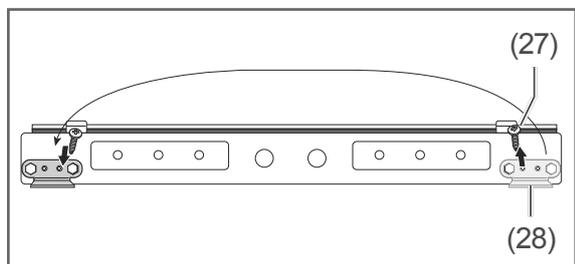
2. Loosen the screw (27) and remove the door fixing (28).
