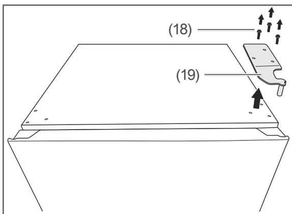
2. Use the cross-tip screwdriver or the 8 mm spanner to loosen the screws (18) and remove the upper hinge (19).
