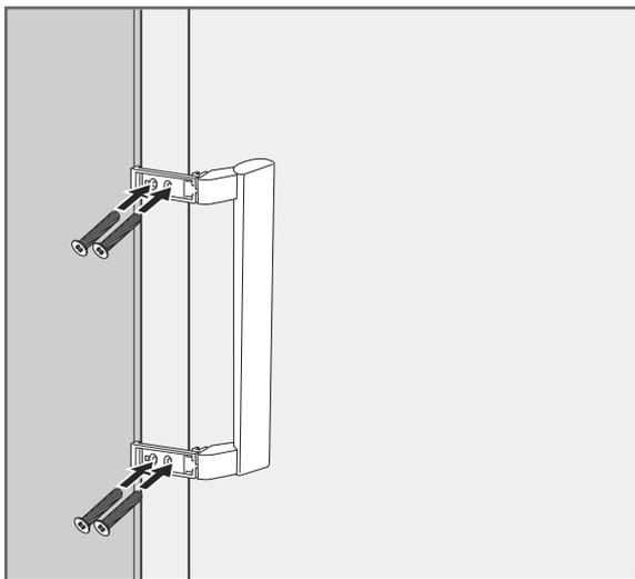
2. Secure the door handle to the appliance door using the four screws provided.
