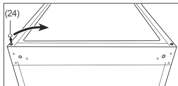
6. Loosen the blind plug (24) on the left side and reinsert it on the right side.
