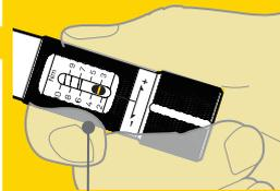
**IMPORTANT NOTE:** Hold the Torq Stick at position shown when applying torque to achieve highest accuracy.
