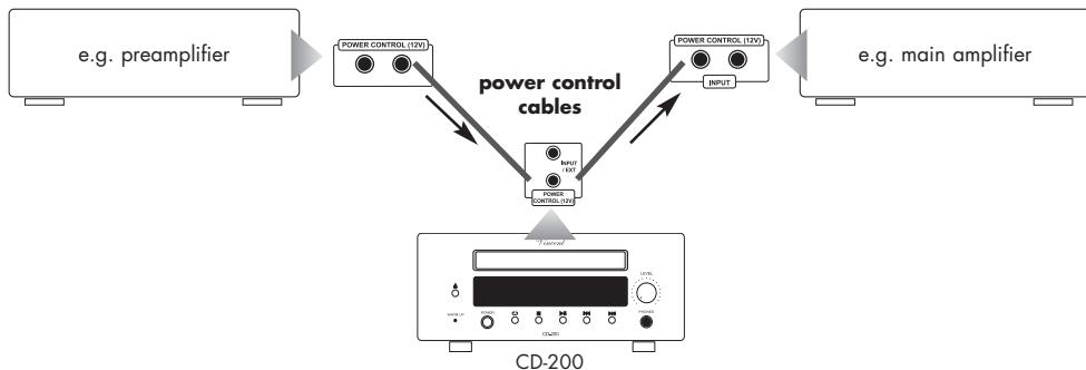
A theoretically infinite number of devices may be served with the switch impulses from a transmitting device. To this end, on most devices one of the two "POWER CONTROL" connectors may be used as a signal input and the other as a signal output. This method of passing on the signal via the devices' inputs and outputs and of thereby chaining them is also known as "daisy chaining".
