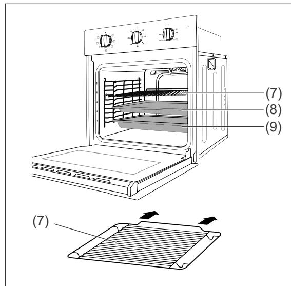
The side walls of the cooking compartment are equipped with baking tray guides (6).
