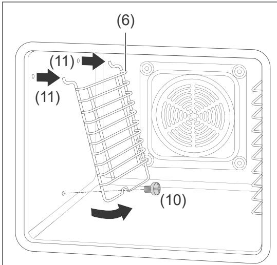
3. Fold up the baking tray guides from below and carefully pull the curved brackets (11) upwards from the wall.
