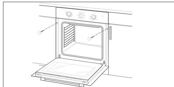
3. Once the oven is correctly positioned, open the oven door and screw into the unit using the fitting screws supplied.
