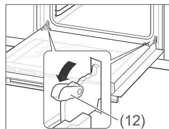
2. Fold the clips (12) on both sides all the way forward. Use a screwdriver if necessary.
