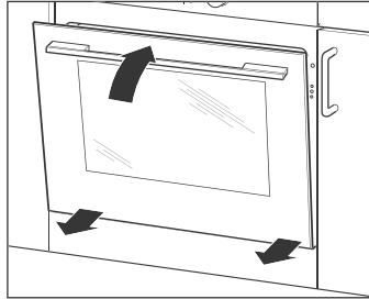
4. Lightly lift and guide the door forward out of its hinges.
