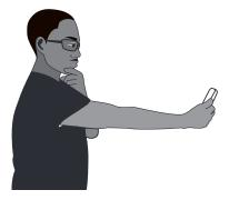
The SPL meter should be held at arm's length, with the microphone pointed at the center point between the left and right speakers (where your head will be), angled at 45 degrees to ensure an accurate reading. If your SPL meter is also your cell phone, make sure your finger or cell phone case isn't covering the mic!
