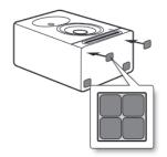
(4) Foam feet to be placed on the bottom of the speaker to improve isolation  $\,$
