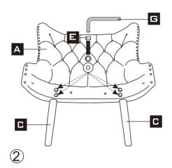
Put the screws in the holes, tight the screws, 100% is ok
