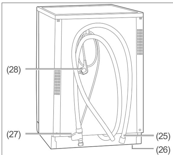
(26) Adjusting feet, 4 (under the machine)
