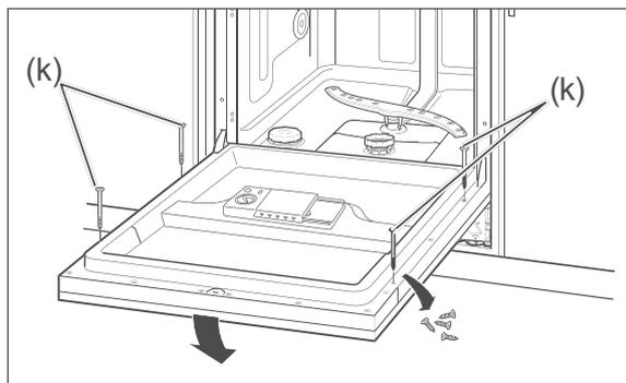
17. Remove the 4 screws from the inside of the door. Screw the front panel at these points using the 4 screws (k) supplied. You have now fitted the front panel.
