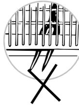
When loading the cutlery, ensure that it does not go through the bottom of the cutlery basket. Otherwise, the lower spraying arm will be blocked.
