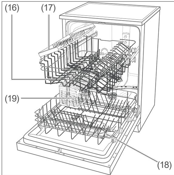
(16) Upper dish rack with the upper wash arm underneath
