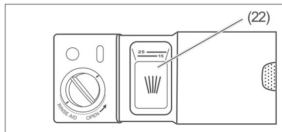
2. Place a multitablet in the dispenser. Push the cover of the compartment closed so that the closure clicks into place once again.
