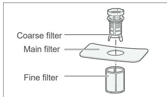
Remove any food scraps out of the coarse filter, the main filter and the fine filter.
