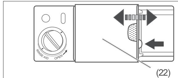
1. Slide the blue fastener on the dishwasher detergent/multitablet dispenser (22) to the side. The cover moves to the side and the dispenser becomes visible.
