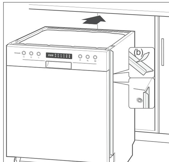
5. Remove the protective films from the side end profiles (b).
