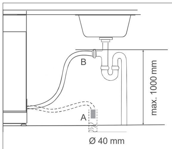
The outlet hose (22) can be connected in two ways:
