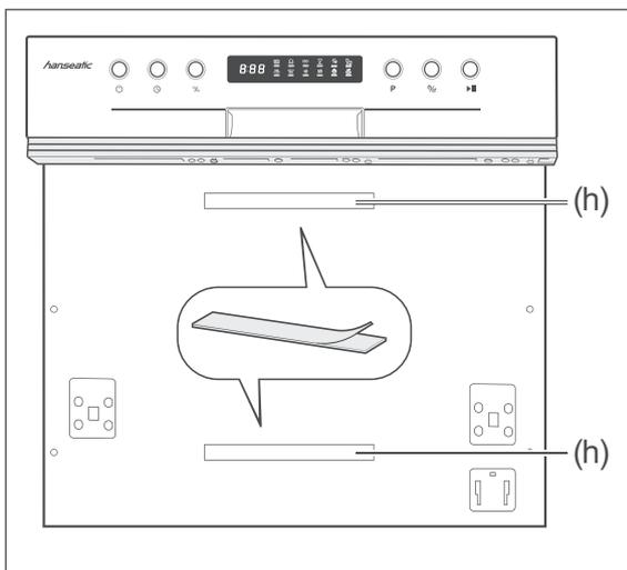
9. With the protective film removed, stick the Velcro strips (h) to the middle of the recessed areas on the dishwasher door.
