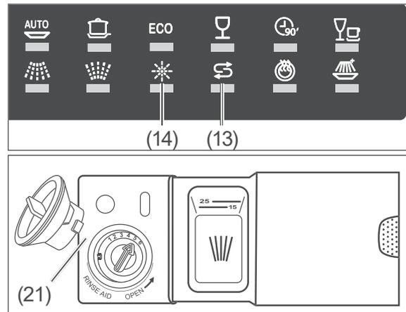
1. Turn the cover of the rinse aid dispenser (21) a quarter of a turn anticlockwise and remove it.
