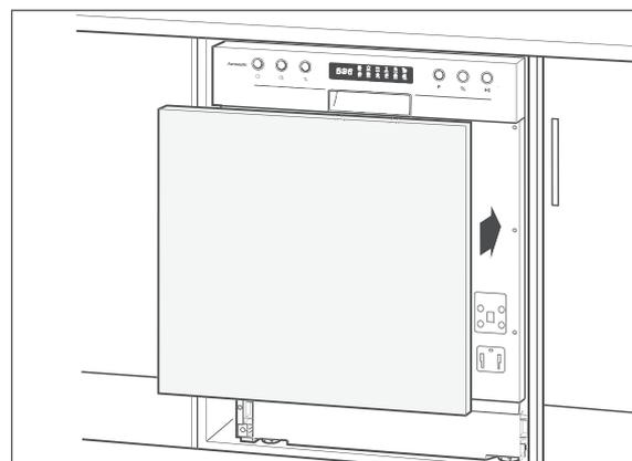
16. Fix the front panel to the dishwasher door using the Velcro strips (h), hold it firmly and carefully open the door.
