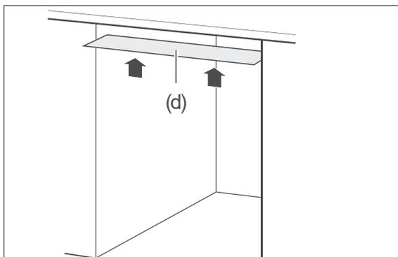
3. Affix the condensation protection film supplied (d) to the underside of the worktop. In this way, you will avoid damage to the worktop as a result of hot steam which may come out of the dishwasher when the door is opened.
