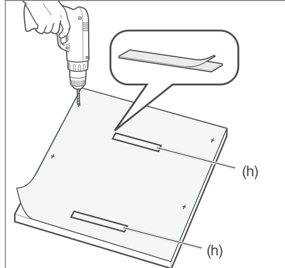
12. Lay the supplied drilling template on the reverse side of the front panel in such a way that the drilling template and the front panel are flush at the top.
