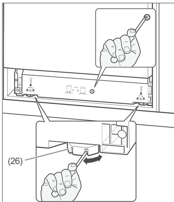
8. To position the dishwasher so that it is level, the two front feet (26) and the back foot on the appliance can be adjusted by up to 50 mm.
