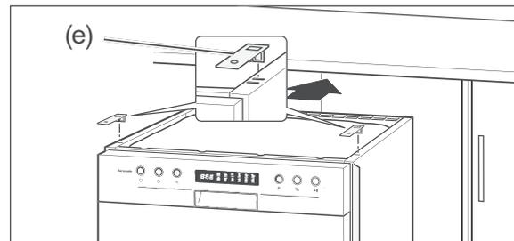
4. Insert the two mounting brackets (e) into the front slots on the top of the dishwasher so that you can screw the dishwasher to the worktop subsequently.
