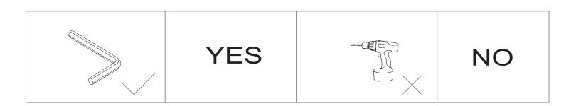
Attention: DO NOT TIGHTEN THE SCREWS UNTIL ALL PARTS ARE IN RIGHT POSITIONS.
