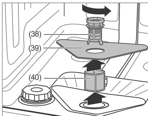
Regularly remove any food scraps from the coarse filter (38), the main filter (39) and the fine filter (40).
