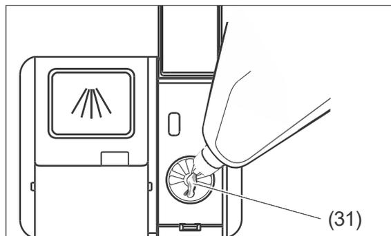
2. Fill the water tank to the “max” mark in the opening.
