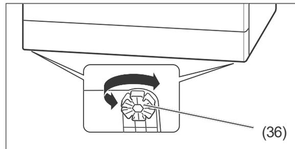
2. To equalise unevenness in the floor and set up the dishwasher on a level horizontal base, you can screw the two adjustable (36) feet in or out. The adjustable feet have slots around their circumference. Insert a screwdriver into one of them and use it to turn the adjustable foot. Use a spirit level to align the dishwasher.
