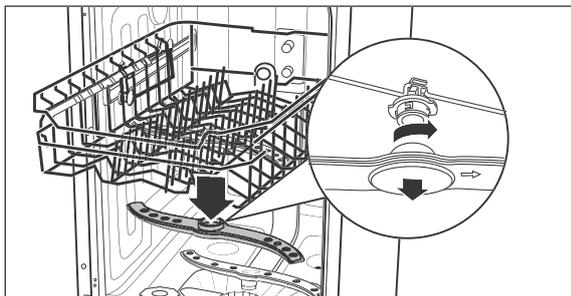
3. The upper spraying arm is affixed using a bayonet closure. In order to remove the spraying arm, hold both of the toothed bayonet holders still and turn the spraying arm in a clockwise direction.
