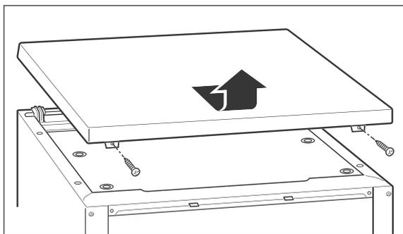
1. Turn the two screws on the back of the cover plate.
