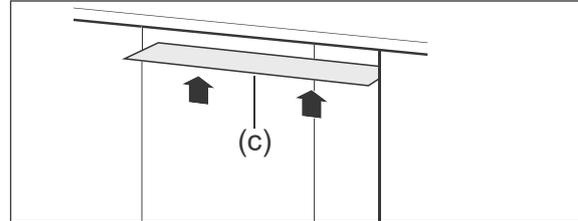
4. Affix the enclosed condensation-protective film (c) to the underside of the work surface. In this way, you will avoid damage to the work surface as a result of hot steam which may be emitted from the dishwasher if the dishwasher door is left open.
