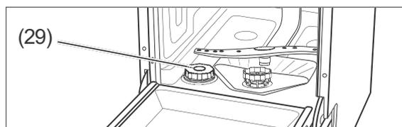
2. Turn the cover of the dishwasher salt dispenser (29) in an anti-clockwise direction and remove it.
