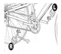
**Note:**Be sure to identify R/L letters on pedal's bolt when you installing.
