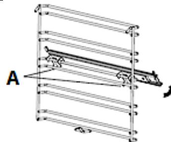
2. Then turn the telescopic slide anti-clockwise slightly (s. fig. on the right, arrow).
