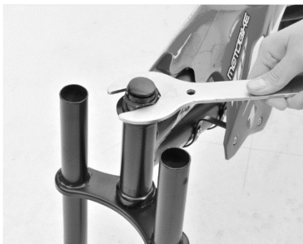
Figure 1: Release Head Tube Nut
