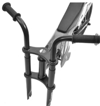
Figure 1: Align handlebars over the fork and head tube
