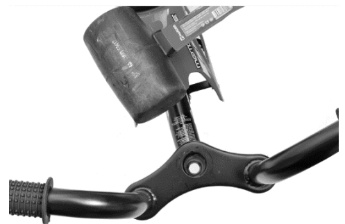
Figure 3: Align Bars on fork and frame.
