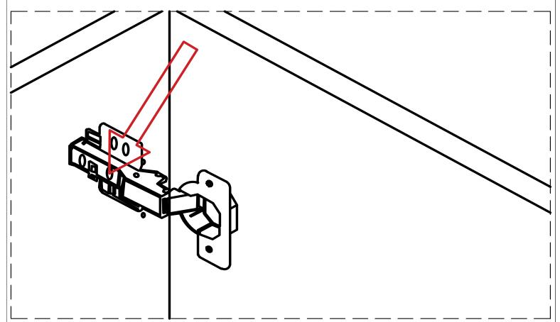
This screw is used to adjust the gap at the bottom of the door panel
