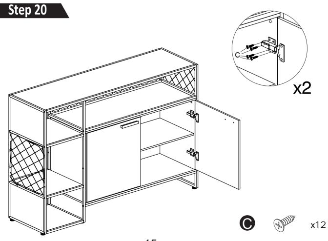
This screw is used to adjust the side clearance of the door panel
